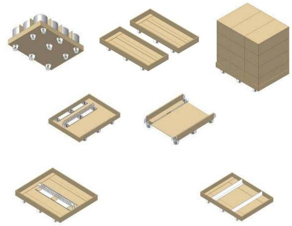
Once the basic design and performance traits of the system are understood, designs can be customized in a near limitless assortment of ways, optimizing the solution for the specific application. Using various internally positioned substrate materials, additional corrugated assemblies, and/or internally assembled corner board, the standard OptiTray can be customized for additional benefits.
