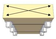
The combination of the packaging and the internal contents (product and dunnage) must be able to withstand strapping and stacking pressures without excessive damage or compression. The increased weight associated with stacking multiple unit loads may cause vertical compression that then loosens previously tight straps. It's imperative that the straps remain taunt to securely hold the OptiLedge devices in place.
