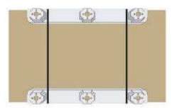
Although it is possible to design intermediary packaging components when configuring an OptiLedge solution for odd-shaped products, it is recommended that geometric friendliness be observed. For the OptiLedge device to work properly, it's critical that it be integral to the unit load by being securely attached to a solid 90° angle of a rigid item across its full length. Lack of support or freedom due to gaps or flexibility can damage the OptiLedge devices and the product.
