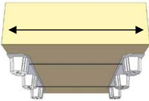
The product/package should be capable of supporting itself in a rigid fashion across spans between OptiLedge devices. It must also be able to withstand interaction with handling equipment across the bottom surface of the unit. If necessary, substrate materials can be used to strengthen the span and the bottom surface.
