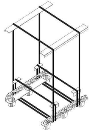
Base-layer strapping is always recommended to minimize strap lengths. Should unit loads of product compress when stacked, (a likely occurrence under heavy weights) base-layer strapping minimizes the amount of slack that could occur within the straps thereby assuring the OptiLedges remain in place. It also ensures a safe base for order picking once the unit load strap is cut. Base-layer sub-assembly is one of the most important keys to building successful unit loads.
