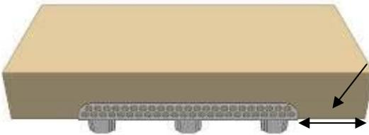
Over-hang is a critical issue when developing an OptiLedge solution and should be carefully considered and tested as necessary. Excessive over-hang, typically greater than 7.5" can cause product deflection at the ends of the unit load. A perimeter solution can often alleviate this. Note that carton corners provide a substantial portion of the unit load stacking strength, and long-term storage may impart forces on the unit load that short-term viewing doesn't always convey.
