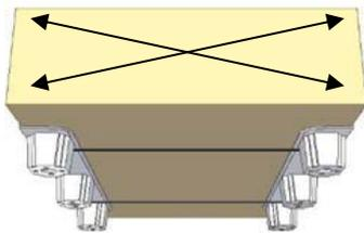
The combination of the packaging and the internal contents (product and dunnage) must be able to withstand strapping and stacking pressures without excessive damage or compression. The increased weight associated with stacking multiple unit loads may cause vertical compression that then loosens previously tight straps. It's imperative that the straps remain taut to securely hold the OptiLedge devices in place.
