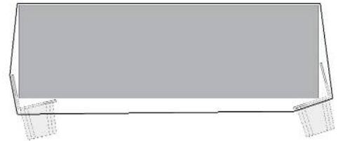
Note that when applying strapping, a minimum of two straps per OptiLedge pair should be used and they should always be positioned as close to the outer feet as possible. In some cases, a third strap, placed on either side of the center foot, may be necessary as well.
