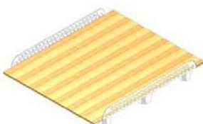
For some products, it may be beneficial to utilize a solid wooden (or other similar material) substrate sheet to provide additional unit load bearing distribution and center support on the underside of the unit loads.
